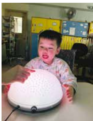
聲控觸覺燈透過感應聲音而發出不同顏色的光，增加學員與環境的互動性 Voice responsive dome provided colour change by sensing sound to enhance the interaction between children and the environment
